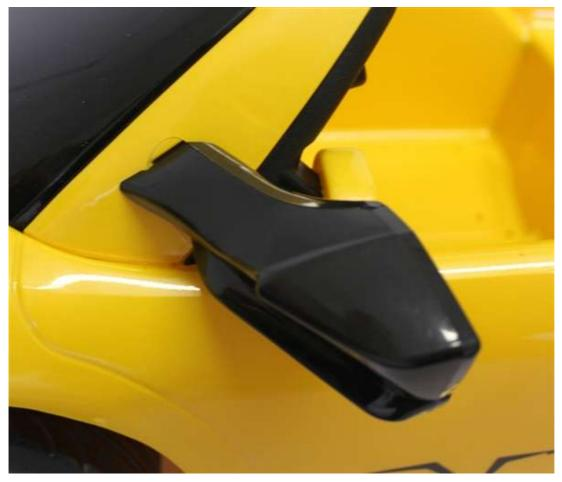
8) Then replace the screw to secure the mirror in place, repeat for both sides.
