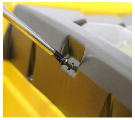
11) Click the seat in to place, and replace the screw to secure it.
