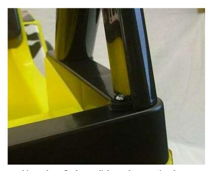
With the rollbar secured in to place, fix the two lights to the top, using the same screws.
