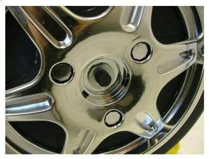
Then to finally fit the wheel in place, have one last check that everything is properly assembled, then push on the wheel securing clip. It will click in to place. Repeat this for both sides. The rear wheels are now secured to the car.
