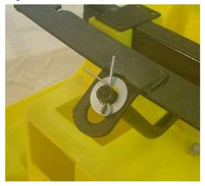
Then, fit the front wheels in the same manner as the rear wheels. Push the wheel on to the steering axle, then a washer, and finally a securing clip to fix the wheel in to place.
