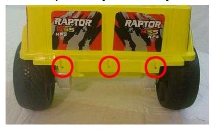
Then place the bumper on the rear of the car, and fix it in place with three screws like this;
