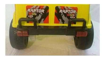
Take the rear rollbar base, and place it on to the top of the rear of the car, noting the four securing screws. These can be fiddly, it's worth shaking the four screws in to place before putting the base on to the car.
