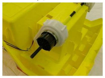
Finally, push on the rear wheel (which has a star shape inside, the front wheels do not have this).
