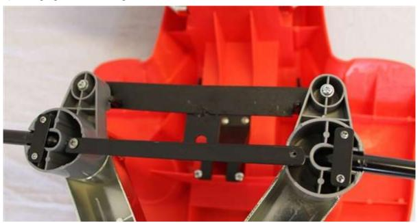
5) And insert the bolt and tighten to match the opposite side. The nut will self lock, it does not need to be tight, else it will prevent the steering from working freely.
