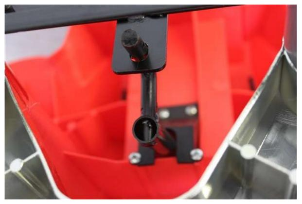
9) Secure with a washer and split pin from the assembly pack.
