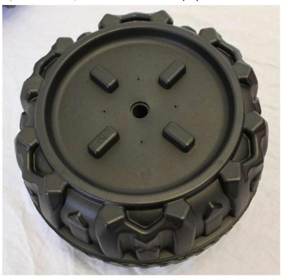
12) Push the wheel centre in to the wheel, repeat on the inside and outside of the front wheels.
