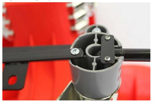
8) Take the steering column and push it down in to the body, then slide it back up in to the steering rack as shown.
