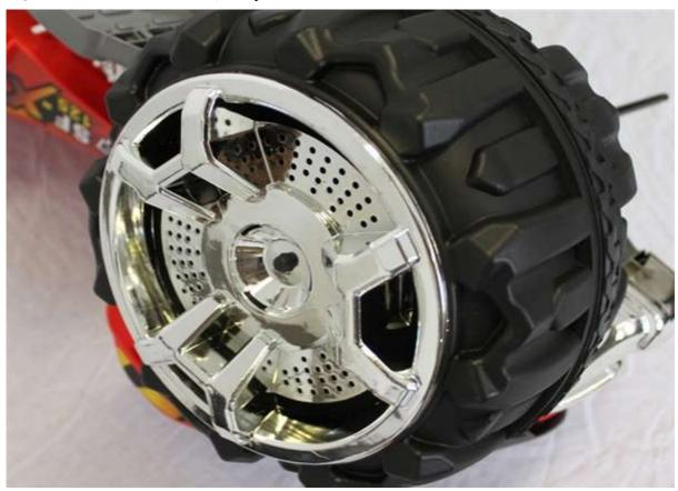
17) Then take a washer and wheel securing nut, and tighten. Do not over-tighten, the wheel nut is self-locking, and over-tightening will prevent the wheels from turning.
