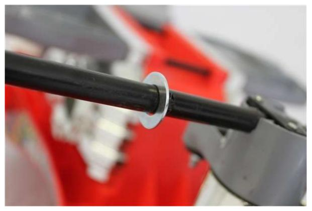
15) Then slide on the wheel, making sure the wheel centres are inserted fully on both the inside and outside (as step 12/13).
